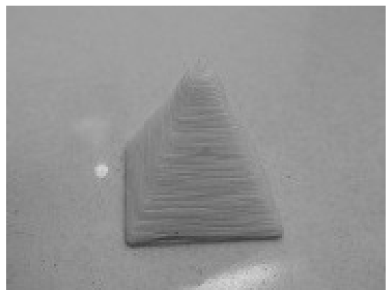
Fig. 6. Poor surface finish due to lines
