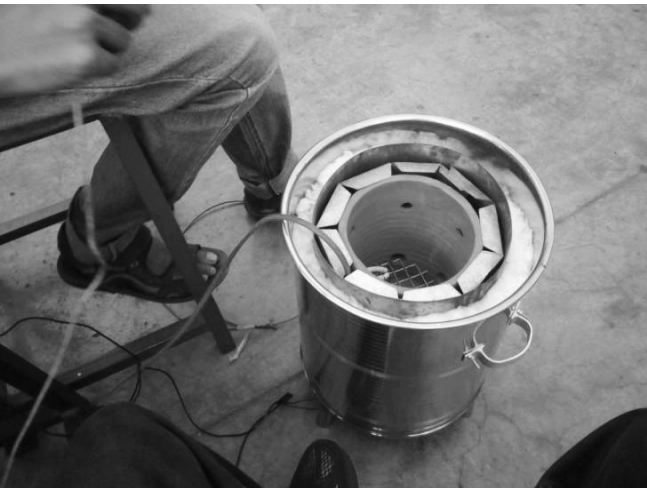
Fig. 2. Stove with thermocouples attached
